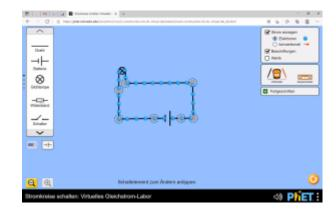
It is also possible to display circuit symbols instead of symbols. Phet.Colorado.edu works with US-American circuit symbols by default. However, it is possible to switch to the display format that is common here in Europe or Germany. To do this, I go to Options in the lower menu bar and select circuit symbols according to standard IEC.
